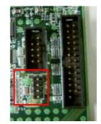
IDEB1: IDE Interface Connector (40Pin 2.54mm Pitch Header)
